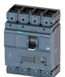
CIRCUIT BREAKER 3VA2 IEC FRAME 400 BREAKING CAPACITY CLASS C ICU=110KA @ 415 V 4-POLE, LINE PROTECTION ETU860, LSIG, IN=250A OVERLOAD PROTECTION IR=100A ...250A SHORT CIRCUIT PROTECTION ISD=0,6..10X IN, II=1,5..12X IN NEUTRAL PROTECTION ADJUSTABLE (OFF, UPTO 160%) GROUND-FAULT, SWITCHABLE IG=0,2... 1 X IN, TG=0,05-0,8MS BUSBAR CONNECTION
