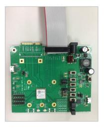
3. Connect the two antennas to the u.FL connectors on the DVK-ST60-SIPT/DVK-SU60-SIPT board.
