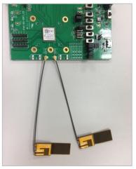
The development board can be powered from a DC 12V supply (into DC jack connector CN1), USB (type micro-B) connector (USB1 and USB2), or the host interface (SDIO interface).
