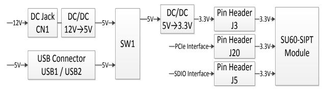
For regular usage, the power from SDIO bus should be enough with no need for external power from either the DC jack or USB port. To run continuous TX in a regulation test, the host may not be able to support enough current via the SDIO and may need external power.
