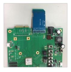
2. Solder each pin of the SDIO extender board.
