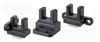
this series of photomicrosensors with Photo-IC output type (Dark-on & Light-on), 3 types of mounting styles, and 2 power supply voltages (5V and 12V). For some specific applications a zener diode can be added on the output of the photomicrosensor to provide greater noise immunity (EE-SX3162-P1-Z and EE-SX4162-P1-Z only).
