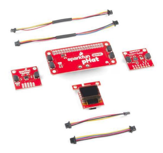
The SparkFun Qwiic Kit for Raspberry Pi includes the Sparkfun Qwiic HAT for Raspberry Pi, which adds four Qwiic connectors to your Pi. It also includes a VCNL4040 Proximity Sensor Breakout, Micro OLED Breakout, Environmental Combo breakout and plenty of Qwiic Cables to connect everything together.
