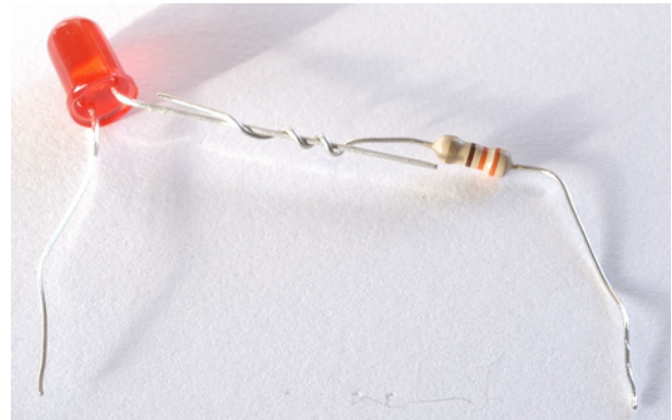
Kinked ends of resistor & LED wires for better connection
