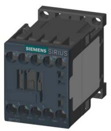
CONTACTOR, AC-3, 4KW/400V, 1NO, AC 24V, 50/60 HZ, 3-POLE, SZ S00 SCREW TERMINAL
