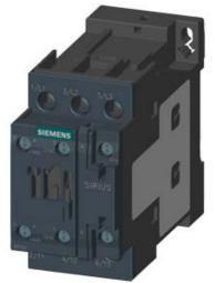
CONTACTOR, AC-3, 5.5KW/400V, 1NO+1NC, DC 48V, 3-POLE, SZ S0 SCREW TERMINAL
