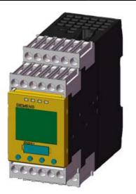
SIRIUS SAFETY RELAY SAFETY-RELATED SPEED MONITORING, 24 V DC, 45.0 MM, SCREW-TYPE CONNECTION, ENABLING CIRCUIT INSTANTANEOUS:2NO, ENABLING CIRCUIT DELAYED: 0, SIGNALING CIRCUIT: 2 ELECTRICAL, NAMUR VERSION, AUTO START / MANUAL START, BASIC UNIT, MAX. ERR. PL EN13849-1: E, MAX. ERR. SIL TO IEC61508:3,
