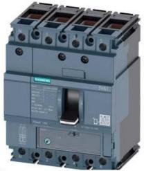
CIRCUIT BREAKER 3VA1 IEC FRAME 160 BREAKING CAPACITY CLASS H ICU=70KA @ 415 V 4-POLE, LINE PROTECTION TM220, ATFM, IN=25A OVERLOAD PROTECTION IR=17,5A ...25A SHORT CIRCUIT PROTECTION II=10 X IN NEUTRAL PROTECTION 100% CABLE CONNECTION
