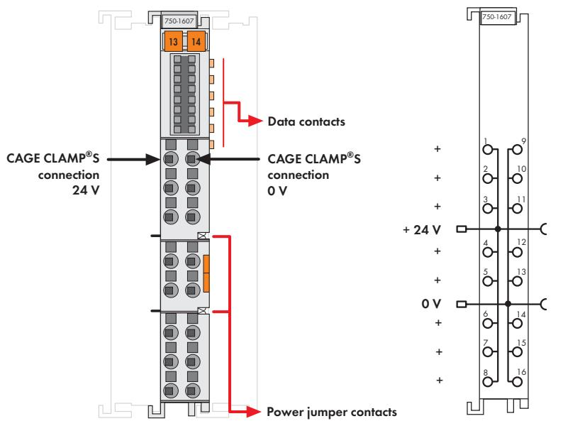
The field side connection module provides 24 V and 0 V power for the inputs and outputs of the 8-channel input/output module 750-1506 (also suitable for 8-channel I/O modules, 1-wire connection) eliminating external terminal blocks.
