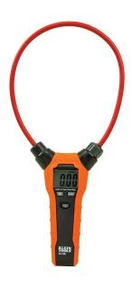
This easy to use, stand-alone meter features an 18" flexible clamp that allows access into panels and hard to reach areas (bundled wires, awkward conductors and PLC cabinets). True RMS readings with CATIV 600V or CATIII 1000V safety ratings. Features Backlit LCD Display, Auto-power Off after 15 minutes, Max/Min, Hold, Auto-Ranging and Low Battery icons.
