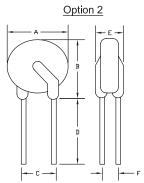
Lead Size : 20AWG Ø0.81mm Diameter
