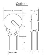
Lead Size : 24AWG ø0.51mm Diameter
