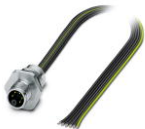
Flush-type connector, Power, 6-position, Plug, M12, M - Power, Front mounting, M16 x 1.5, Individual wires, cable length: 0.2 m
