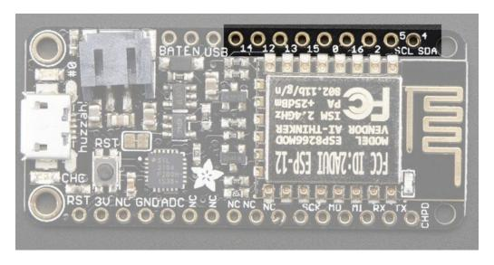
This breakout has 9 GPIO: #0, #2, #4, #5, #12, #13, #14, #15, #16 arranged at the top edge of the Feather PCB
