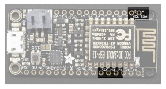
In theory you can use *any* pins for I2C and SPI but to make it easier for people using existing Arduino code, libraries, sketches we set up the following:
