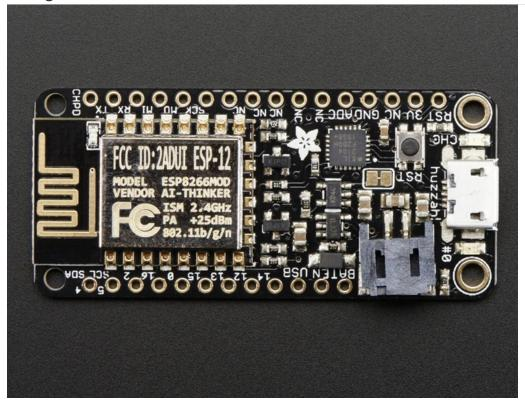
While the Feather HUZZAH ESP8266 comes pre-programmed with NodeMCU's Lua interpretter, you don't have to use it! Instead, you can use the Arduino IDE which may be more familar. This will write directly to the firmware, erasing the NodeMCU firmware, so if you want to go back to Lua, use the flasher to re-install it
