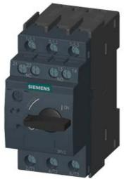
CIRCUIT-BREAKER SZ S00, FOR MOTOR PROTECTION, CLASS 10, A-RELEASE 7...10A, N-RELEASE 130A, SCREW CONNECTION, STANDARD SW. CAPACITY W. TRANSVERSE AUX. SWITCH 1NO+1NC
