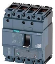
CIRCUIT BREAKER 3VA1 IEC FRAME 160 BREAKING CAPACITY CLASS N ICU=25KA @ 415 V 4-POLE, LINE PROTECTION TM240, ATAM, IN=20A OVERLOAD PROTECTION IR=14A ...20A SHORT CIRCUIT PROTECTION II=5...10 X IN NEUTRAL UNPROTECTED BUSBAR CONNECTION
