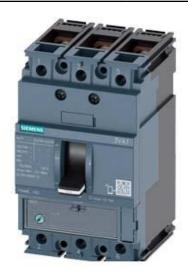
CIRCUIT BREAKER 3VA1 IEC FRAME 160 BREAKING CAPACITY CLASS S ICU=36KA @ 415 V 3-POLE, LINE PROTECTION TM220, ATFM, IN=25A OVERLOAD PROTECTION IR=17,5A ...25A SHORT CIRCUIT PROTECTION II=12,8 X IN BUSBAR CONNECTION
