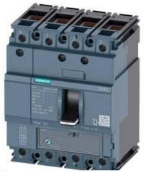
CIRCUIT BREAKER 3VA1 IEC FRAME 160 BREAKING CAPACITY CLASS H ICU=70KA @ 415 V 4-POLE, LINE PROTECTION TM220, ATFM, IN=16A OVERLOAD PROTECTION IR=11,2A ...16A SHORT CIRCUIT PROTECTION II=10 X IN NEUTRAL UNPROTECTED CABLE CONNECTION
