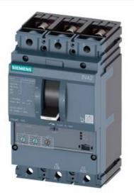
CIRCUIT BREAKER 3VA2 IEC FRAME 160 BREAKING CAPACITY CLASS C ICU=110KA @ 415 V 3POLE, LINE PROTECTION ETU320, LI, IN=40A OVERLOAD PROTECTION IR=16A ...40A SHORT CIRCUIT PROTECTION II=12 X IN BUSBAR CONNECTION
