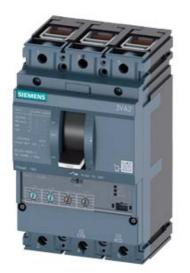
CIRCUIT BREAKER 3VA2 IEC FRAME 160 BREAKING CAPACITY CLASS C ICU=110KA @ 415 V 3POLE, LINE PROTECTION ETU350, LSI, IN=40A OVERLOAD PROTECTION IR=16A ...40A SHORT CIRCUIT PROTECTION ISD=1,5... 10 X IR, II=12 X IN CABLE CONNECTION
