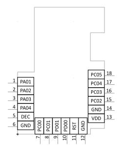
Figure 6.1. MGM210L Lighting Module Pinout
