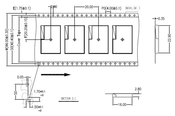
Figure 10.1. Carrier Tape Dimensions
