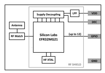
Figure 3.1. MGM210L Block Diagram
