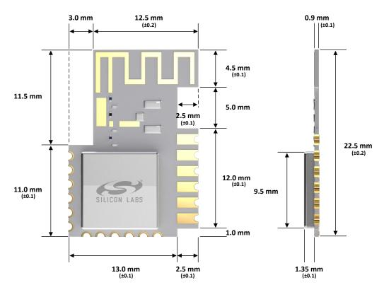
Figure 8.1. Module Dimensions
