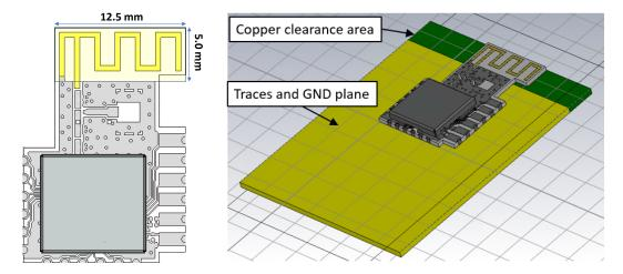
Figure 7.1. Inverted-F Antenna Clearance
