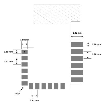
Figure 8.2. Recommended Module PCB Land Pattern
