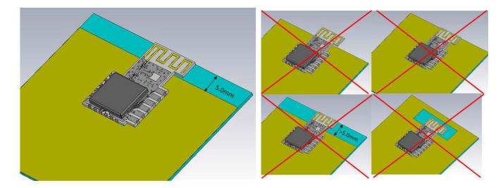
Figure 7.2. Horizontal Mounting
