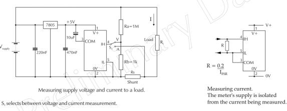
Ra and Rb shown scaled for 200V<sub>FSR</sub> Rs = 200 mV (e.g.  $0.1\Omega/400 mW$  for 2A full scale)  $I_{\scriptscriptstyle \mathsf{FSR}}$ Display DP1, DP2 or DP3, by connecting to 0V, as required.
