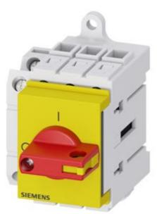
Switch disconnector 3LD3, main switch 3-polig, lu 40A operational switch at AC-23 A at 400 V 15,0 kW Distribution board mounting Base mounting with knob-operated mechanism red/yellow with auxiliary 1NO+1NC
