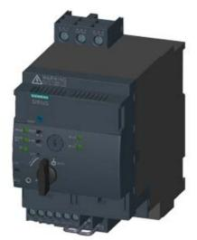
SIRIUS, COMPACT STARTER, REVERSING STARTER . 690 V, 24 V DC, 0.1 ... 0.4 A, IP20, CONN. MAIN CIRCUIT: SCREW TERMINAL, CONN. CONTROL CIRCUIT: SCREW TERMINAL
