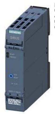
Thermistor motor prot. relay Standard evaluation unit 22.5 mm enclosure Spring-type terminals 2 CO contacts US = 24 V AC/DC Manual/Auto/Remote RESET with ATEX certification 2 LEDs (READY/TRIPPED) Protective separation Test/Reset button Open-circuit monitoring Short-circuit monitoring Non-volatile
