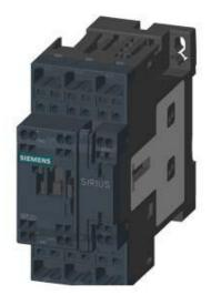
CONT. F. RAILW. A., AC-3, 18.5KW/400V, 1NO+1NC, . DC 72 V, 0,7...1,25\*US, W. VARISTOR INTEGRATED, 3-POLE SIZE S0, SPRING-LOADED TERMINAL
