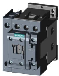
2NO+2NC CONTACTOR, AC3: 11KW AC 24V 50HZ 4-POLE, 2NO+2NC, SZ: S0, SCREW TERMINAL 1NO+1NC INTEGR.
