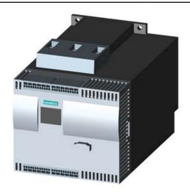
SIRIUS SOFT STARTER, VALUES WITH 575 V, 50 DEG., STANDARD: 51A, 40HP, INSIDE-DELTA CIRCUIT 3: 88A, 75HP, 400-690 V AC, 115 V AC, CAGE CLAMP TERMINALS
