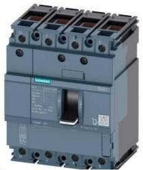
CIRCUIT BREAKER 3VA1 IEC FRAME 160 BREAKING CAPACITY CLASS S ICU=36KA @ 415 V 4-POLE, LINE PROTECTION TM210, FTFM, IN=20A OVERLOAD PROTECTION IR=20A FIXED SHORT CIRCUIT PROTECTION II=10 X IN NEUTRAL PROTECTION 100% CABLE CONNECTION
