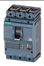
CIRCUIT BREAKER 3VA2 IEC FRAME 100 BREAKING CAPACITY CLASS M ICU=55KA @ 415 V 3POLE, LINE PROTECTION ETU860, LSIG, IN=100A OVERLOAD PROTECTION IR=40A ...100A SHORT CIRCUIT PROTECTION ISD=0,6..10X IN, II=1,5...12X IN NEUTRAL PROTECTION OPTIONAL WITH EXT. CT,UPTO 160% GROUNDFAULT, SWITCHABLE IG=0,2... 1 X IN, TG=0,050,8MS CABLE CONNECTION
