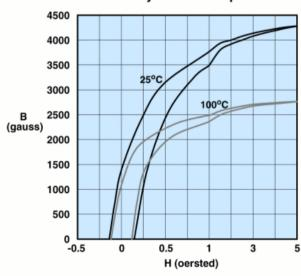
Measured on a 17/10/6mm toroid at 10kHz.
