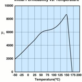
Measured on a 17/10/6mm toroid at 10kHz.
