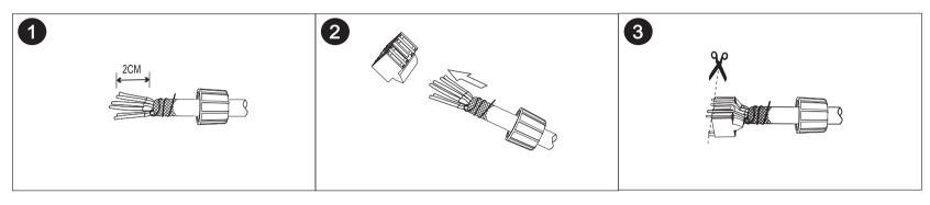
Strip 2cm of cable jacket and wrap earth wire around jacket.
