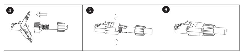
Push cable and core carrier onto the PCB.
