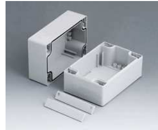
C2108121 ROBUST-BOX 80 BREIT, Ausf. I ABS (UL 94 HB) lichtgrau RAL 7035 120x80x80mm IP 66
