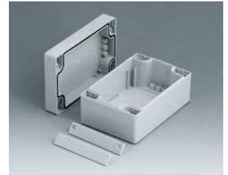
C2008122 ROBUST-BOX 80 BREIT, Ausf. II PC (UL 94 HB) lichtgrau RAL 7035 120x80x60mm IP 66
