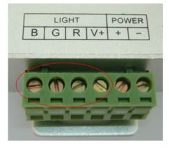
Colour coded screw terminals for LED strip.
