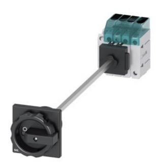
Switch disconnector 3LD3, main switch 3-polig + N, lu 25A operational switch at AC-23 A at 400 V 9,0 kW floor mounting Base mounting with door coupling center-hole 22,5 mm rotary operationg mechanism black  $66 \times 66$  mm with auxiliary 1NO+1NC
