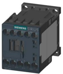
CONTACTOR, AC-3, 5.5KW/400V, 1NO, AC110V 50HZ, 120V 60HZ 3-POLE, SZ S00 SCREW TERMINAL
