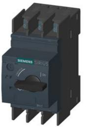
CIRCUIT-BREAKER SZ S00, FOR MOTOR PROTECTION, CLASS 10, A-REL. 1.4...2A, N-RELEASE 26A, RING CABLE LUG CONNECTION STANDARD SW. CAPACITY
