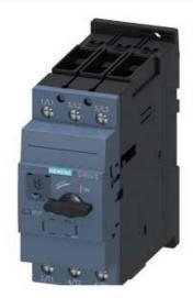
CIRCUIT BREAKER, SIZE S2, FOR TRANSFORMER PROTECTION, A-RELEASE 22...32A, N-RELEASE 640A, SCREW TERMINAL, STANDARD BREAKING CAPACITY
