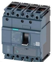
CIRCUIT BREAKER 3VA1 IEC FRAME 160 BREAKING CAPACITY CLASS H ICU=70KA @ 415 V 4-POLE, LINE PROTECTION TM220, ATFM, IN=125A OVERLOAD PROTECTION IR=87,5A ...125A SHORT CIRCUIT PROTECTION II=10 X IN NEUTRAL UNPROTECTED BUSBAR CONNECTION
