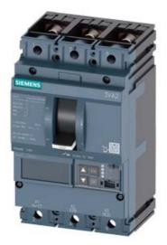
CIRCUIT BREAKER 3VA2 IEC FRAME 160 BREAKING CAPACITY CLASS M ICU=55KA @ 415 V 3POLE, LINE PROTECTION ETU550, LSI, IN=160A OVERLOAD PROTECTION IR=64A ...160A SHORT CIRCUIT PROTECTION ISD=0,6..10X IN, II=1,5..10X IN NEUTRAL PROTECTION OPTIONAL WITH EXT. CT,UPTO 160% BUSBAR CONNECTION
