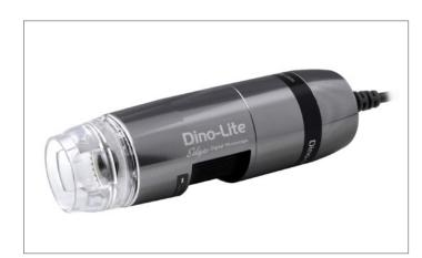
The AM7515MT8A is a 5MP Dino-Lite Edge Series microscope that has a magnification range of700-900x with built-in coaxial illumination. By using the Flexible LED Control (FLC), this model is capable of switching between or mixing, brightfield and coaxial illumination.
