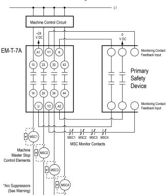
Generalized EM-T-7A Wiring for Two-Channel Control
