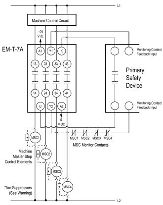
One-channel control affords simplicity of wiring. However, one-channel wiring requires eliminating the possibility of an unsafe failure of the control wires (which connect the output of the Primary Safety Device to the input of the Extension Module).
