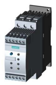
SIRIUS SOFT STARTER, S0, 32A, 15KW/400V, 40 DEGR., AC 200-480V, AC/DC 24V, SCREW TERMINALS, THERMISTOR MOTOR PROTECTION
