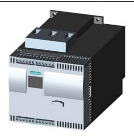
SIRIUS SOFT STARTER, VALUES WITH 460 V, 50 DEG., STANDARD: 26A, 15HP, INSIDE-DELTA CIRCUIT 3: 45A, 30HP, 200-460 V AC, 115 V AC, SCREW TERMINALS
