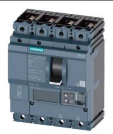
CIRCUIT BREAKER 3VA2 IEC FRAME 160 BREAKING CAPACITY CLASS L ICU=150KA @ 415 V 4POLE, LINE PROTECTION ETU560, LSIG, IN=160A OVERLOAD PROTECTION IR=64A ...160A SHORT CIRCUIT PROTECTION ISD=0,6..10X IN, II=1,5..10X IN NEUTRAL PROTECTION ADJUSTABLE (OFF, UPTO 100%) GROUNDFAULT, SWITCHABLE IG=0,2... 1 X IN, TG=0,050,8MS BUSBAR CONNECTION
