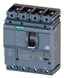
CIRCUIT BREAKER 3VA2 IEC FRAME 160 BREAKING CAPACITY CLASS M ICU=55KA @ 415 V 4POLE, LINE PROTECTION ETU320, LI, IN=40A OVERLOAD PROTECTION IR=16A ...40A SHORT CIRCUIT PROTECTION II=12 X IN NEUTRAL PROTECTION ADJUSTABLE(OFF,100%) BUSBAR CONNECTION
