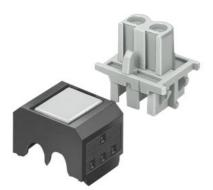
AS-Interface accessory Connection plug for data and auxiliary power line with 2 insulation displacement terminations for standard stranded wires 2 x 0.5...0.75 mm2 flat, yellow, extender
