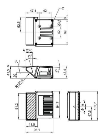
A Optical axis B Deflection angle of the laser beam:  $\pm\,30\,^\circ$
