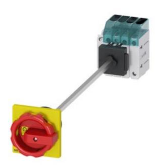
Switch disconnector 3LD3, main switch 3-polig + N, lu 25A operational switch at AC-23 A at 400 V 9,0 kW floor mounting Base mounting with door coupling center-hole 22,5 mm rotary operationg mechanism red/yellow 66 x66 mm with auxiliary 1NO+1NC
