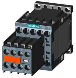
CONTACTOR RELAY, 6NO+2NC, AC 220V 50HZ / 240V 60HZ, SIZE S00, SCREW TERMINAL, PERMANENT AUX. SWITCH, FOR SUVA APPLICATIONS
